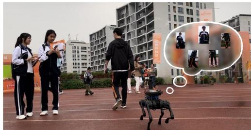
Fig. 1. Robot person following with online continual learning. To this end, long-term and short-term experiences are utilized to optimize the feature extractor online to represent the discriminative appearance of the target person.
