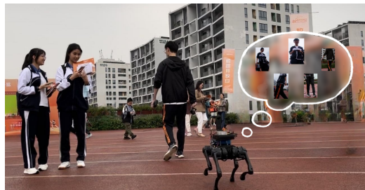
Fig. 1. Robot person following with online continual learning. In this end, long-term experiences are utilized to learn a complete and discriminative appearance model of the target person.
