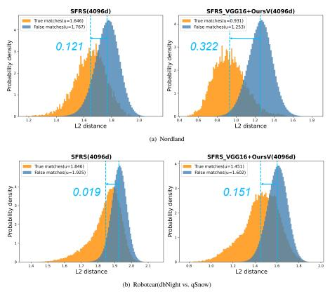
**Figure 6.** L2 distribution of true and false matches for different methods. In both datasets, SFRS\_VGG16+OursV (4096d) surpass SFRS a lot with difference of mean value of 0.322 versus 0.121 in Nordland and 0.151 versus 0.019 in RobotCar (dbNight vs. qSnow).
