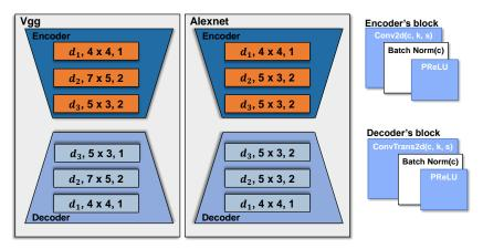
**Figure 3.** The architecture of our CAE. Every encoder block contains Conv2d, Batch Normalization and PReLU layer. In the decoder block, Conv2d is replaced with ConvTranspose2d. c, k, s in the picture means channels, kernel size and stride, respectively.  $d_3$  is a changeable parameter of the last convolutional kernel channels of the encoder, to produce the global descriptor with variable dimensions.
